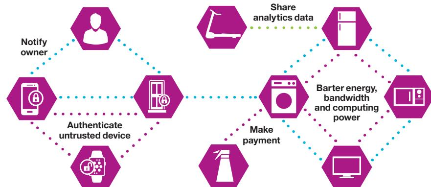
*Peer-to-peer messaging in a decentralized IoT must support: trustless, encrypted messaging and transport; low latency with guaranteed delivery; and storage and forwarding of messages with “hop-on” to other connected devices.*
